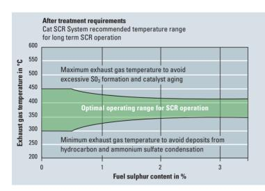
To avoid deposit buildup and ensure optimal operation of the SCR module, the exhaust gas temperature has to be adjusted to the operating conditions for each application.
