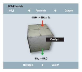
The Cat SCR System is based on selective catalytic reduction technology. A urea solution is injected into the hot exhaust gas and transformed to  $NH_3$  and  $CO_2$ . Inside the SCR module the  $NH_3$  reacts with the  $NO_x$  to form harmless nitrogen and water vapor, which are major components of ambient air.
