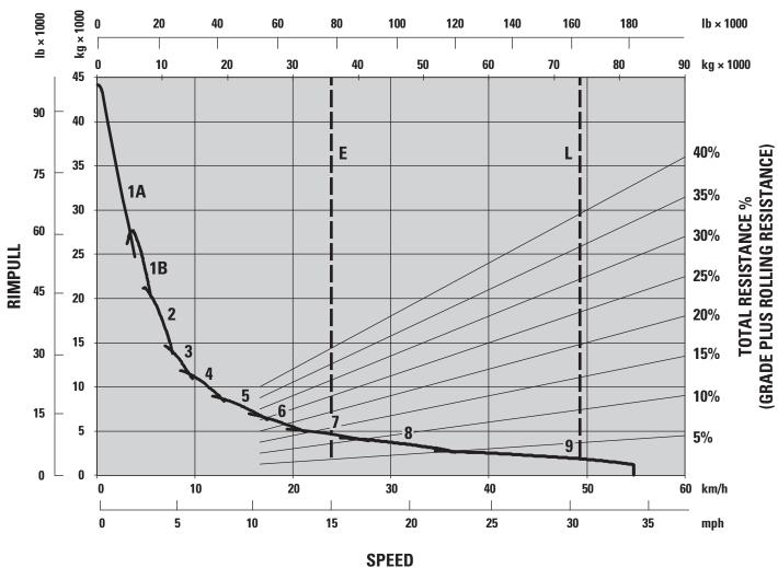
1A – 1st Gear (Converter Drive)
