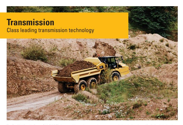
The Cat High Density Power Shift (HDPS) nine-speed forward two-speed reverse transmission, designed specifically for Articulated Trucks, features Advanced Productivity Electronic Control Strategy (APECS) and Electronic Clutch Pressure Control (ECPC) that deliver smooth gear changes with improved acceleration and higher productivity.
