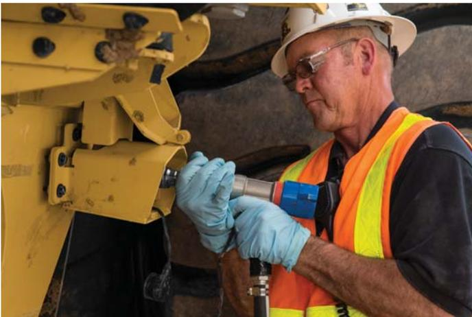
Technician is shown using the ground level DEF fill on a 785G.
