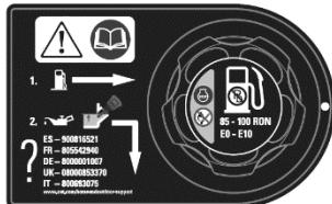
Be alert! Read the Owner's Manual before starting the unit. You must add fuel and oil before starting the unit.
