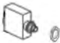
The circuit breaker is held to the panel with a half nut located on the front of the panel. Tag the wires to identify them and then disconnect the circuit breaker. Remove the half nut from the front of the panel then remove the circuit breaker from the rear of the panel.
