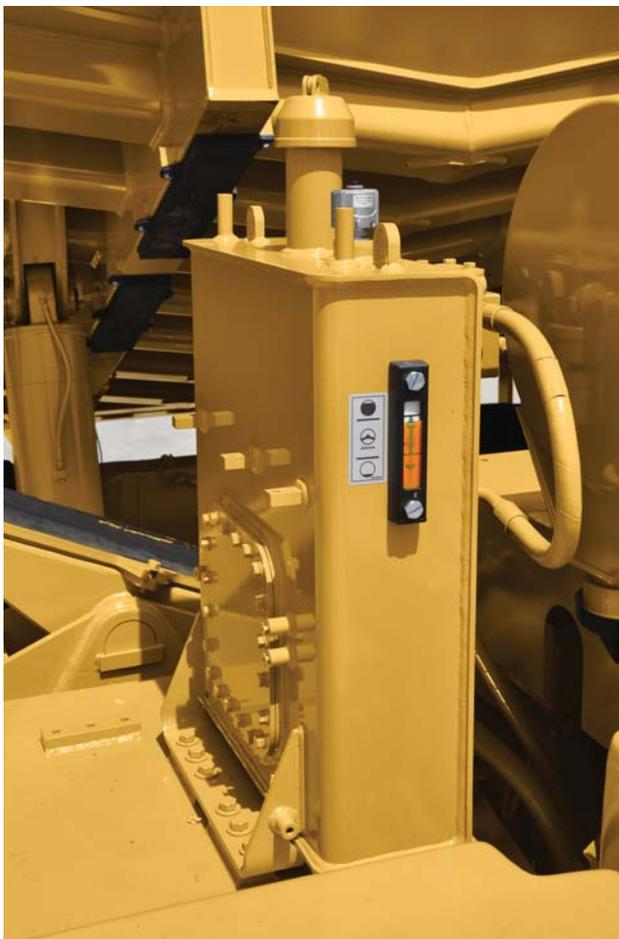
Easy access to daily service points simplifies servicing and reduces time spent on regular maintenance procedures. Enhanced serviceability and extended service intervals are designed to increase machine availability and productivity.
