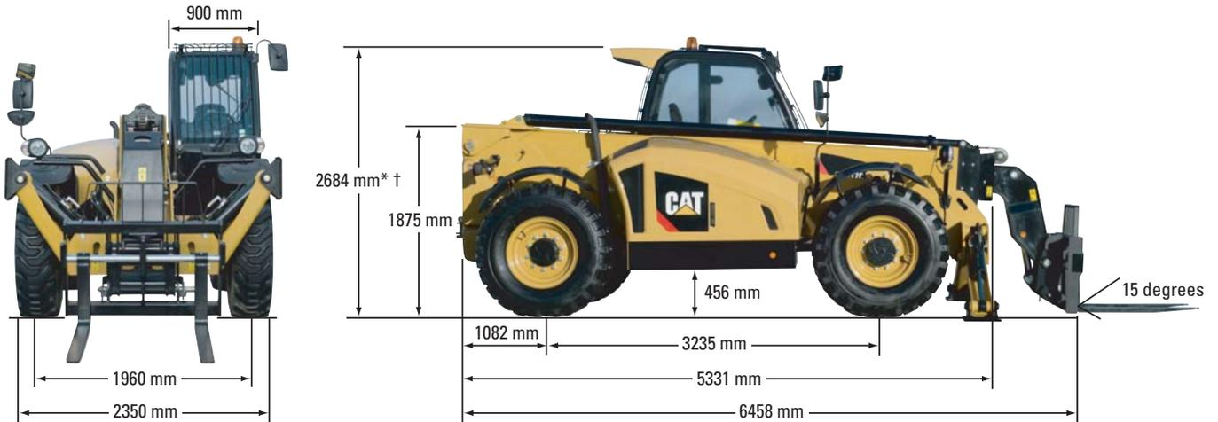
\*to overall height add for the following options: 67 mm for roof guard, 25 mm for air conditioning, 182 mm for beacon
