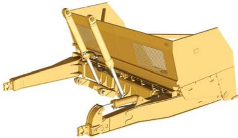
Both scoops come with dual lift cylinders for increased lift capacity. Integrated stabilizer system makes sure that the scoop stays stable and centralized on the machine. Scoop tilt function is standard and provides  $\pm 15$  degrees of tilt to maintain grade conditions and keep your operation safe.
