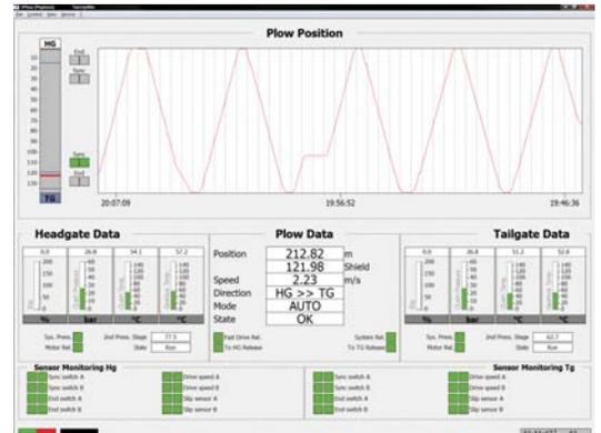
**VPlow** – Visualizes a plow system with solenoid switches and setting of the parameters of the UEL drive controllers.
