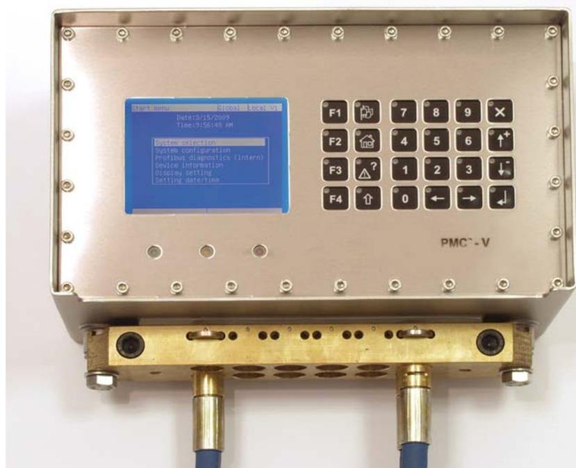
The PMC-V display shows all data available from the gearboxes. This includes all sensor values, status information, all global and local parameters, network status, etc. The change of parameters is easily possible with the 24-key numerical keypad. Important system parameters are password protected.
