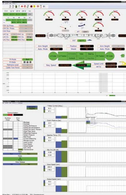
**VDrive** – Visualizes the conveyor gearbox controllers. A range of sensor values can be displayed graphically and all parameters can be changed.
