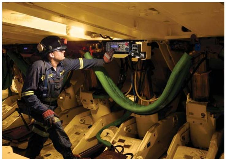
*PMC controllers are protected by stainless steel housings to withstand harshest conditions underground*
