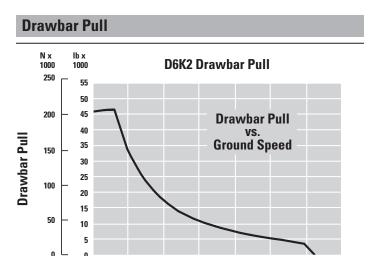
• The direct injection electronic fuel system provides a controlled fuel delivery increase as the engine lugs back from rated speed. This results in increased horsepower below rated power. A combination of increased torque rise and maximum horsepower improves response, provides greater drawbar pull and faster dozing cycles.
