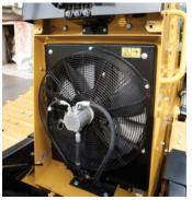
The engine radiator, Air To Air After Cooler (ATAAC), and hydraulic oil cooler are packaged in a single plane. Aluminum bar plate construction provides durability and allows for higher heat transfer and superior corrosion resistance.
