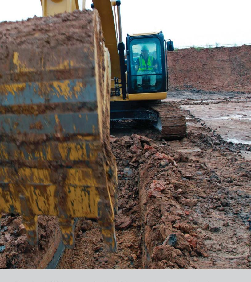
The new Cat 320D2 GC hydraulic excavator is engineered for low owning and operating costs, simple routine maintenance, high productivity and long-term durability. Equipped with a four-cylinder, turbocharged Cat C4.4 ACERT engine, the new model is exceptionally fuel efficient; the fuel saving is up to 17%, compared with 320D2. Fuel saving results may vary depending on applications, conditions, operator behavior, and other external factors.
