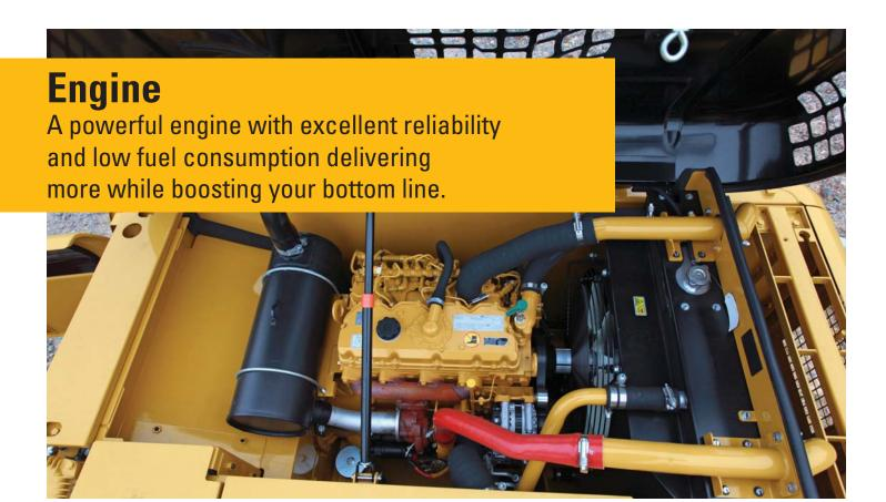
The Cat C4.4 ACERT engine with four cylinders meets Brazil emissions regulation MAR-1. The proven C4.4 ACERT engine incorporates robust components and precision manufacturing you can count on for reliable and efficient operation. Less sensitive to low quality fuel, it boasts improved reliability while delivering reduced fuel consumption.
