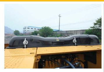
**Anti-skid plating** covers the entire upper structure and storage box to prevent slipping during maintenance. Safety is further enhanced with the addition of countersunk bolts to reduce trip hazards.
