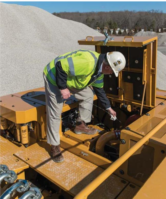
Machine's slip-resistant 500 mm wide catwalks stretch the length of the machine to provide safe access to major and grouped service points, such as fuel and oil filters, and fluid taps.
