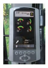
temperature. It is equipped with warning lamp and buzzer for critical warnings, such as issues with engine oil pressure, coolant temperature, and oil temperature. Filters and fluid change intervals are available in the main menu. Machine information in the event display is in the form of both text and icon. The multi-informational display exhibits various information that is convenient for the operator in up to 42 languages.
