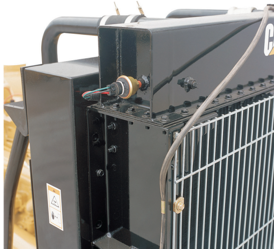
Figure 8: Coolant Level Sensor in a Cat® G3406 Engine
