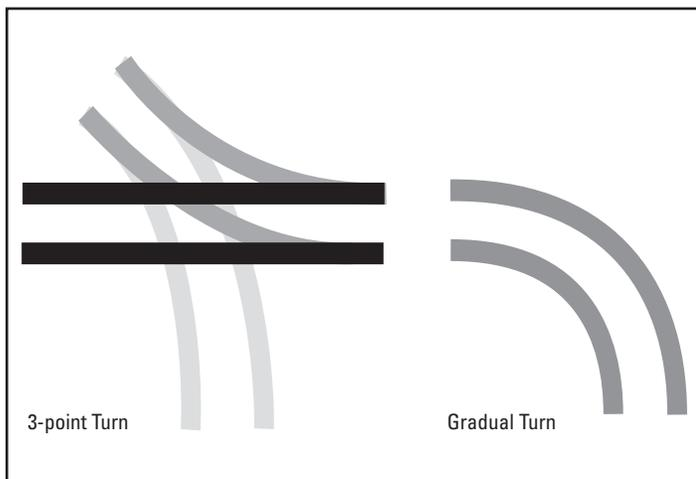
To help maximize the life of a compact track loader undercarriage, counter-rotations should be used only when required, such as in very confined areas. Instead, use more gradual, or 3-point, turns while slowly moving in forward or reverse.
