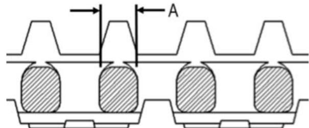
If track forging is less than 34 mm, the track should be replaced.
