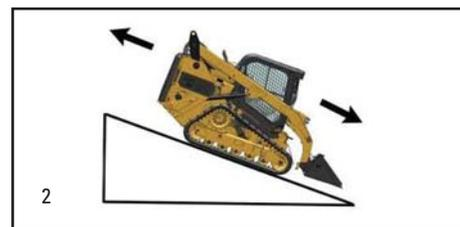
Avoid making direct 90-degree turns when operating on a slope—either on a side hill or straight up and down. Sharp turns on slopes can cause unnecessary wear on track guides (tabs) and can shove material between the track and roller wheels. In some cases, this could lead to track derailment and track damage.
