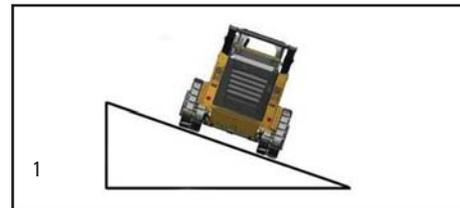
When working up and down a slope (Illus. 2), always keep the heaviest end of the machine uphill. Loaders are typically heavier on the front end of the machine when fully loaded and heavier on the rear end when unloaded. You should also avoid unusually heavy loads and always keep loads as low as possible. Consult the Operation and Maintenance Manual for proper machine operation on slopes.
