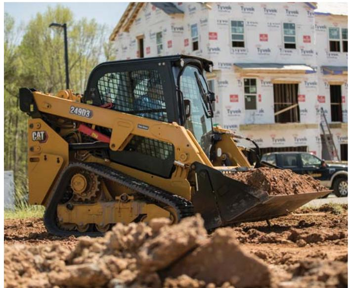
Keeping the full length of track on the ground provides the most traction and takes advantage of the machine suspension. You can get excellent results and maximize the life of your undercarriage by backdragging with loader arms, using the FLOAT function. If more down pressure is needed, the CTL suspension system will allow for additional down pressure to be applied without raising the undercarriage off of the ground. Add only the pressure required to smooth the surface.
