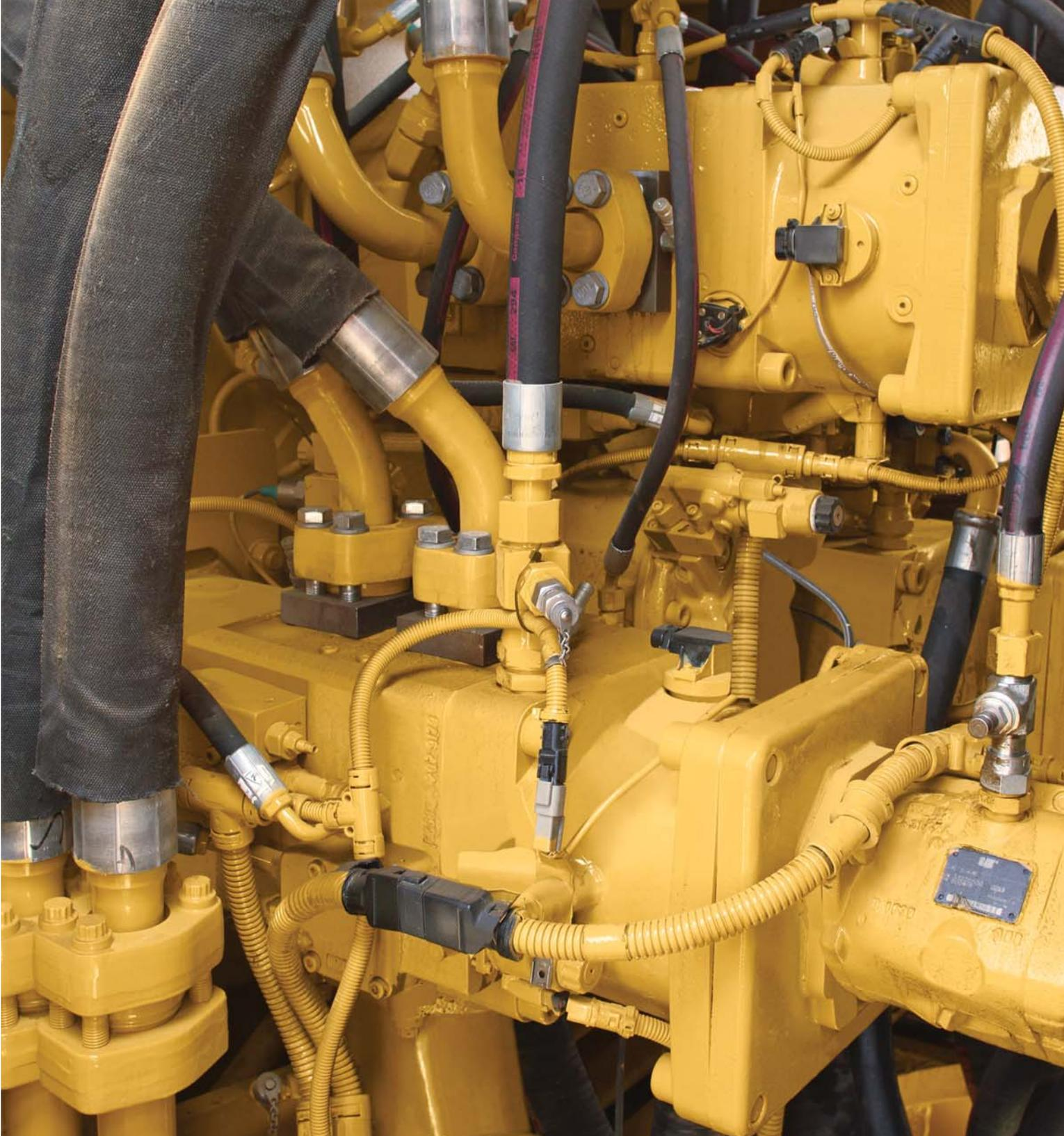
The revolutionary Adaptive Hydraulic System combines industry-leading and patent-pending dedicated pump-flow allocation technology with proven Cat features like independent oil cooling and boom float to generate flow and pressure, without waste – providing a 20% fuel efficiency advantage.
