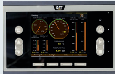
Fig. 13-9 DCU (display and alarm system)
