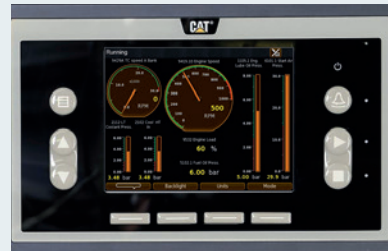
Fig. 13-9 DCU (display and alarm system)
