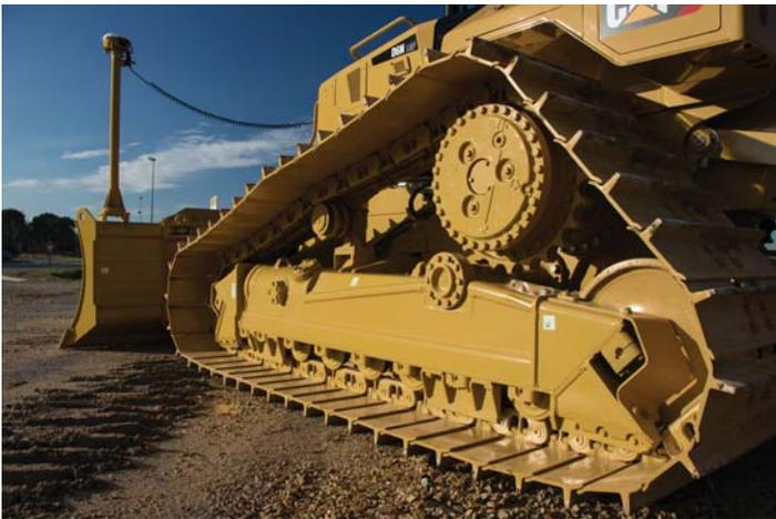
Semi-Universal and Straight blades are designed with a strong box section to stand up to the most severe applications. Heavy moldboard construction, hardened bolt-on cutting edges and end bits add strength and durability.
