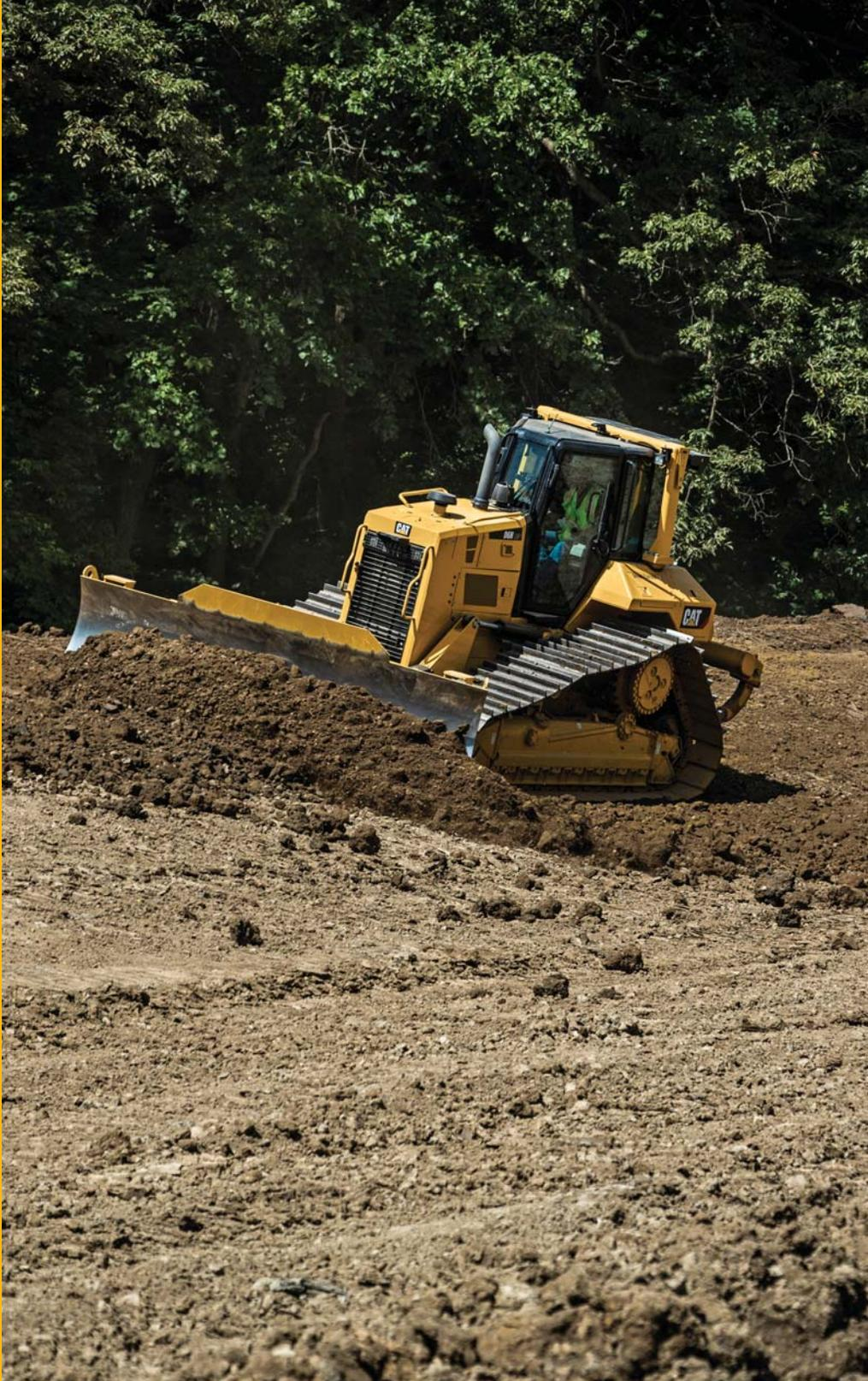
**The latest in the line of Cat D6N dozers combines well-known versatility with a range of technology features to give you more job site productivity than ever before. A new transmission with lock-up clutch torque converter delivers ease of operation, increased net power, plus a 10-15 percent improvement in fuel efficiency. The D6N has the weight and horsepower you want for dozing applications and the balance and stability you need for finish grading – all in one easy-to-transport machine.**
