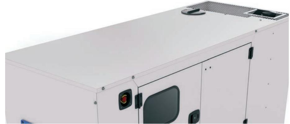
The robust main roof features a flush-mounted rain cap with compression seal, allowing access to the radiator fill whilst providing protection against water ingress.
