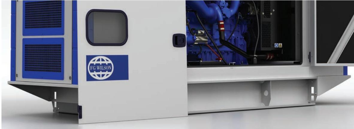
Side hinged doors, on each side of the enclosure, provide ample access to all necessary components during installation and servicing. Lift-off hinges allow doors to be removed, even at an angle of 45°, facilitating servicing in the most confined installation spaces.
