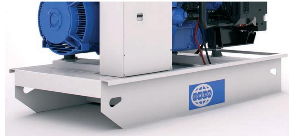
Providing lifting points as standard, aiding transportation and installation, the compact tank base is designed for 8 hours running at full load in prime applications.
