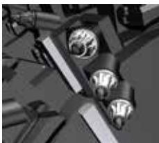
Triple-tree cutting bit placement on rotor ends cleans up loose material and reduces wear on the rotor caused by maneuvering in the cut.
