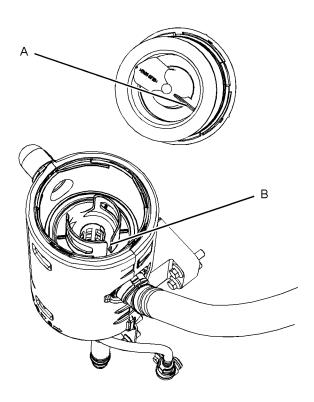
**5.** Install a new filter element into the breather body (3). Ensure the correct position of the element, refer to illustration 94. Align position (A) on the top cap to position (B) on the filter element.
