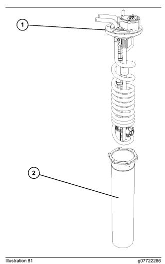
2. Remove outer filter (2) from DEF manifold (1).
