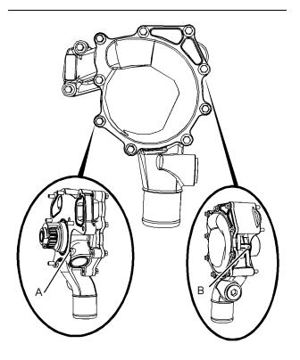
**Note:** The water pump seals are lubricated by the coolant in the cooling system. It is normal for a small amount of leakage to occur. Refer to illustration 95 for the position of the weep hole and the vent hole.
