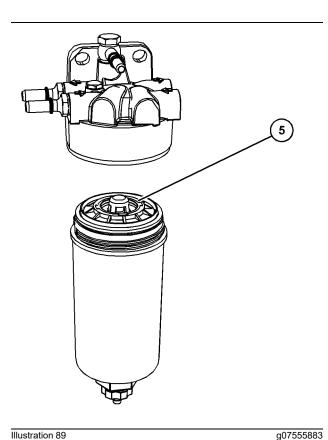
**7.** Rotate the filter element (5) counterclockwise and remove the filter element. Clean the filter bowl.
