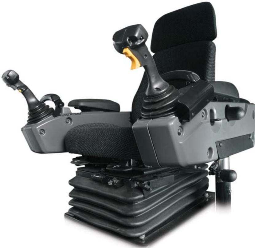
Operators are more comfortable and productive with two electro-hydraulic joysticks. New and experienced operators around the world report that the controls are easy to learn, and that the new electronically adjustable control pods make it easier to position them for optimal comfort, visibility and proper operation.
