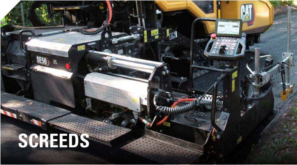
Cat screeds provide excellent durability, easy adjustment, and simple maintenance. Simple heating element replacement and machined screed frames facilitate quick service and reduce operating costs.
