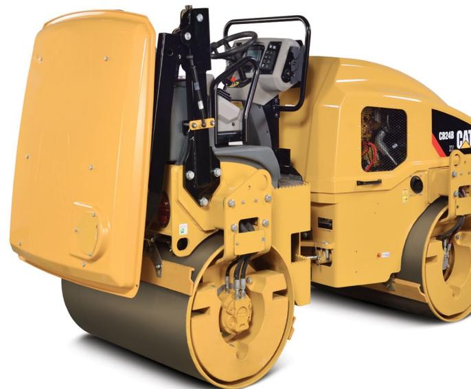
*Jobsites vary, and so do the demands placed on your compactors. Multiple frequency and ballast choices enable the compactor to perform in a variety of conditions, while features such as extra-wide drums and pneumatic tire options enhance production and precision.*
