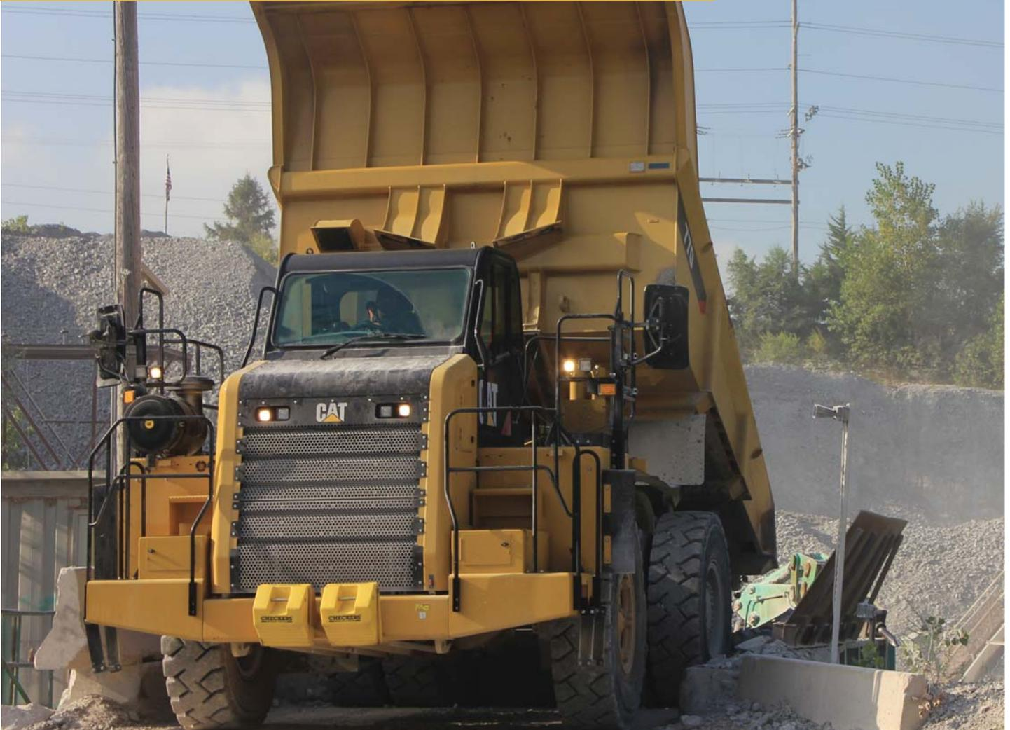
The goal of our body designs is to provide rated payloads on each haul. Since no two jobsites are alike, we offer two body designs, optional sideboards for lightweight materials, and two liner options for the Flat Floor body to protect your investment and achieve the best possible wear life.
