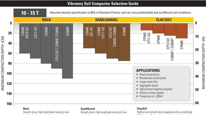
amplitude when approaching compaction, 4-8 passes
