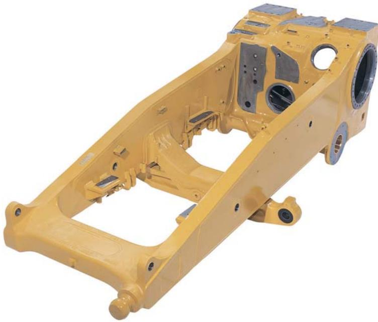
The D8T mainframe is built industry-leading tough – heavy steel castings, full box section frame rails and continuous rolled sections on top and bottom frame rails provide the strength to absorb high impact shock loads and twisting forces.
