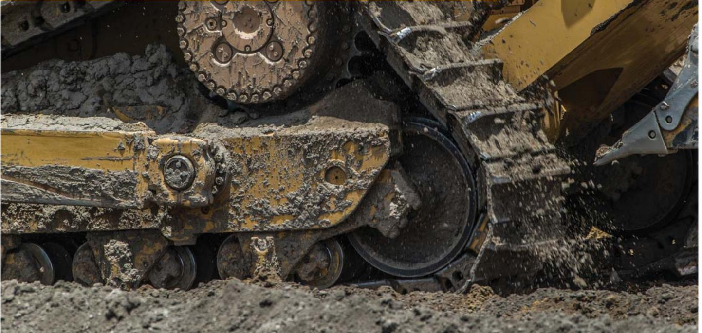
The elevated sprocket and suspended undercarriage work together, increasing traction while creating a smoother ride for your operators. The elevated sprocket design transfers implement shock loads to the mainframe, so final drives, axles and steering components are isolated from harsh impacts. These benefits translate into higher production and longer component life.
