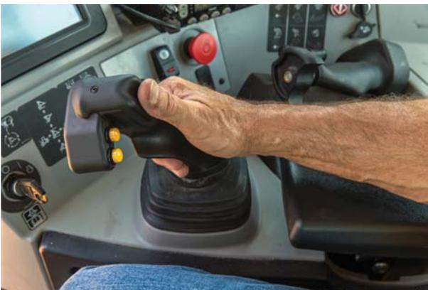
A low-effort electronic dozer control handle gives the operator complete control of all dozer functions with one hand.
