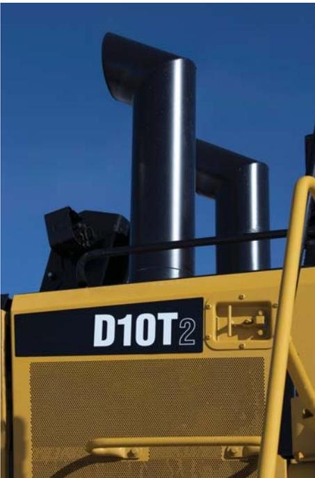
The D10T2 is offered with two variations of the C27 engine with ACERT Technology. One will meet Tier 4 Final emission standards and will be required for sale in higher regulated countries. The other option will be capable of achieving levels equivalent to Tier 2 and Stage II emission standards for lesser or non-regulated countries.
