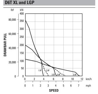
**NOTE:** Usable pull will depend upon weight and traction of equipped tractor.
