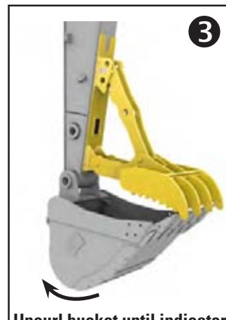
Uncurl bucket until indicator shows pin holes are aligned.
