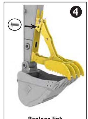
Replace link positioning pin.
