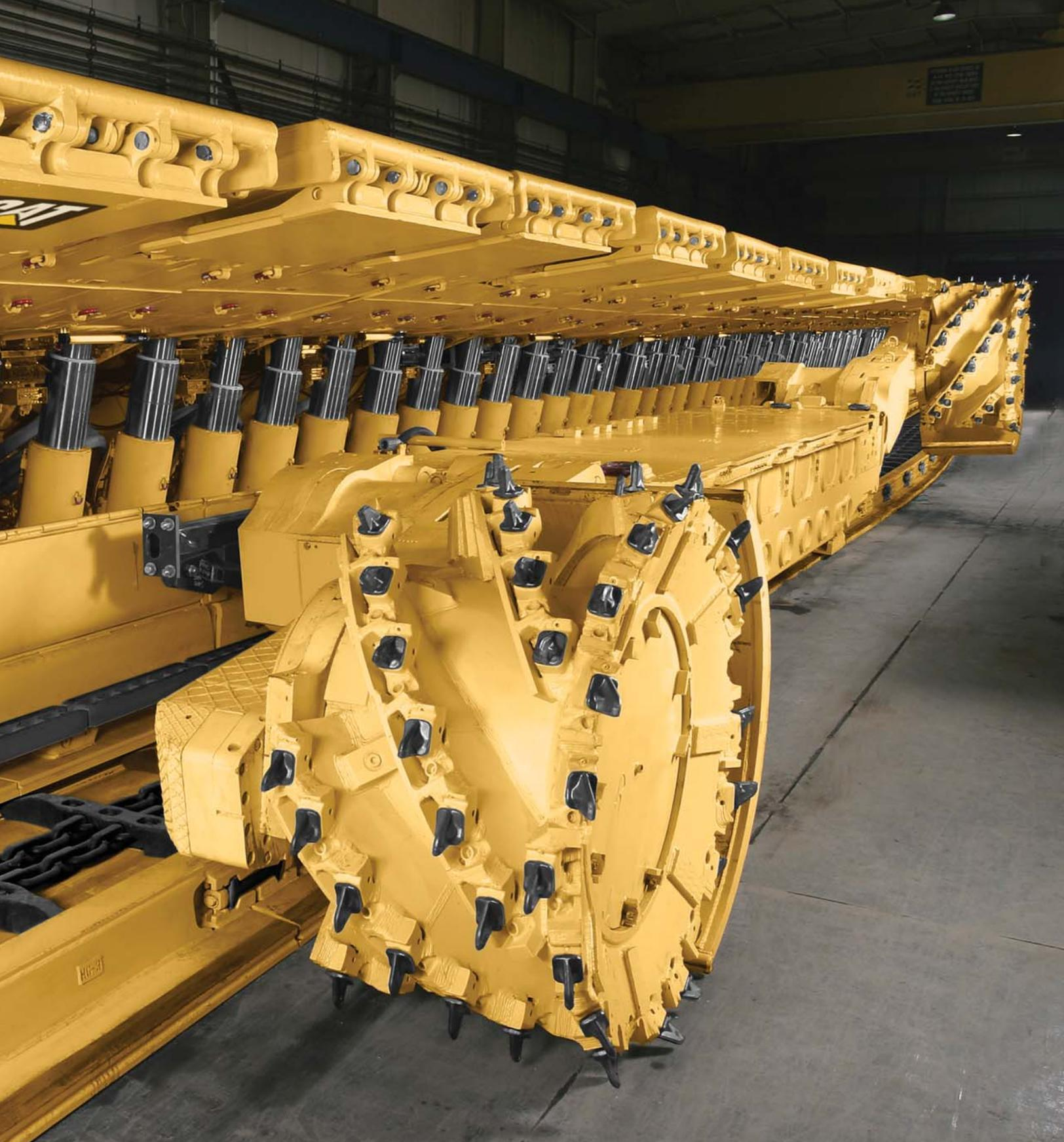
**The EL3000 Shearer has been developed for medium to high seams to meet the requirements of the most demanding longwall installations in the world. The EL3000 mines seams of up to 5.50 m (217 in). It offers 2 × 860 kW (2 × 1,380 hp @ 60 Hz) of cutting power combined with haulage motors of up to 2 × 150 kW (2 × 200 hp), with a 75 kW (120 hp @ 60 Hz) pump motor. With installed power of over 2000 kW (3,600 hp @ 60 Hz) it has a production capacity of more than 5000 tonnes (5,512 tons) per hour.**
