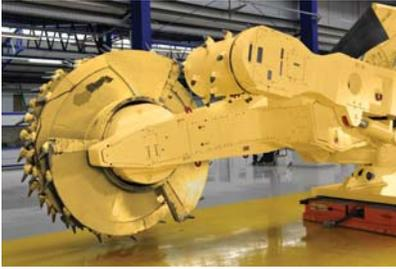
Cat shearers can be supplied with an optional rugged coal sizer, currently with up to 200 kW (268 hp) of installed power for maximum productivity in high seams or difficult mining conditions. The coal sizer can be ordered separately for installation during rebuild or overhaul.
