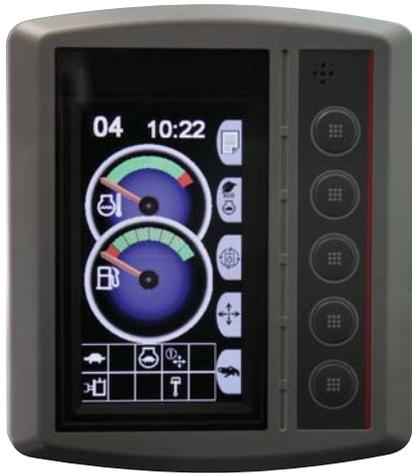
The COMPASS control panel on the Cat E Series mini hydraulic excavators was specifically designed by Caterpillar for compact excavators. It adds several new features to the machines increasing the amount of customer value. All of the following features are now standard on all E Series models.
