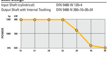
GEARBOX RATIO i [-] Rated Power P [hp] @ 60 Hz Rated Power P [kW] @ 50 Hz
