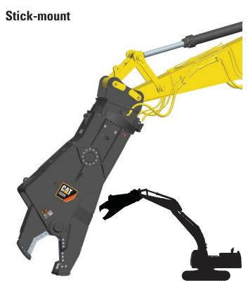
Cat Shears are commonly stick-mounted for use in demolition applications where reach is critical.
