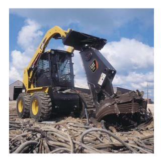
The S305 Mobile Scrap and Demolition Shear, mounted on a mini-excavator or skid steer loader is a very productive tool in processing of lighter steel or non-ferrous material such as cable, rebar, small beams and small diameter pipe.
