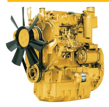
The Cat 3054CA engine has been designed to meet U.S. EPA Tier 2 and EU Stage II emission regulations. This engine incorporates a time-proven mechanical governor and a low-pressure fuel injection system that are major contributors to the improvement of fuel system robustness, high fuel efficiency, and ease of troubleshooting. High filtration performance from the primary filter incorporating a water separator and a secondary filter also help to improve fuel filtration system reliability.
