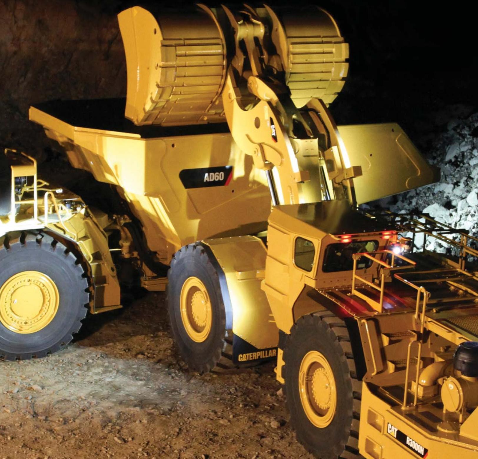
**The AD60 Underground Articulated Truck is designed for high production, low cost-per-ton hauling in underground mining applications. Rugged construction and simplified maintenance guarantee long life with low operating costs.**
