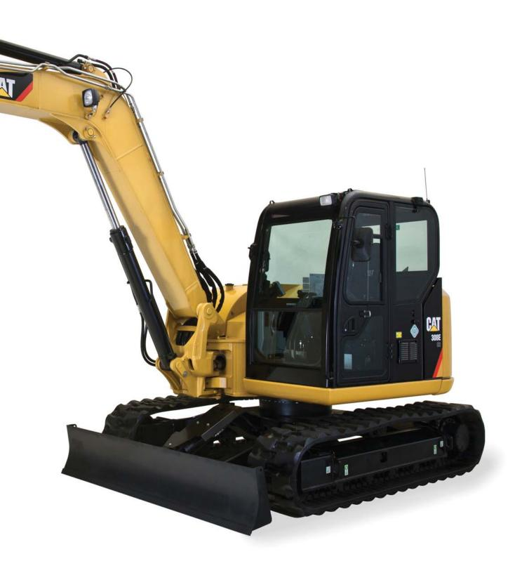
The Cat® 308E CR SB Mini Hydraulic Excavator delivers high performance with the versatility of a swing boom front linkage in a durable Compact Radius design to help you work in the tightest applications. With the new COMPASS display panel and redesigned operator environment, the 308E CR SB is more productive, versatile, and cost effective.
