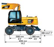
\*\* Maximum tire clearance with outrigger fully down
