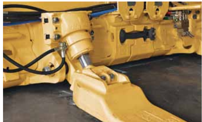
Horizon control for easy height adjustments
