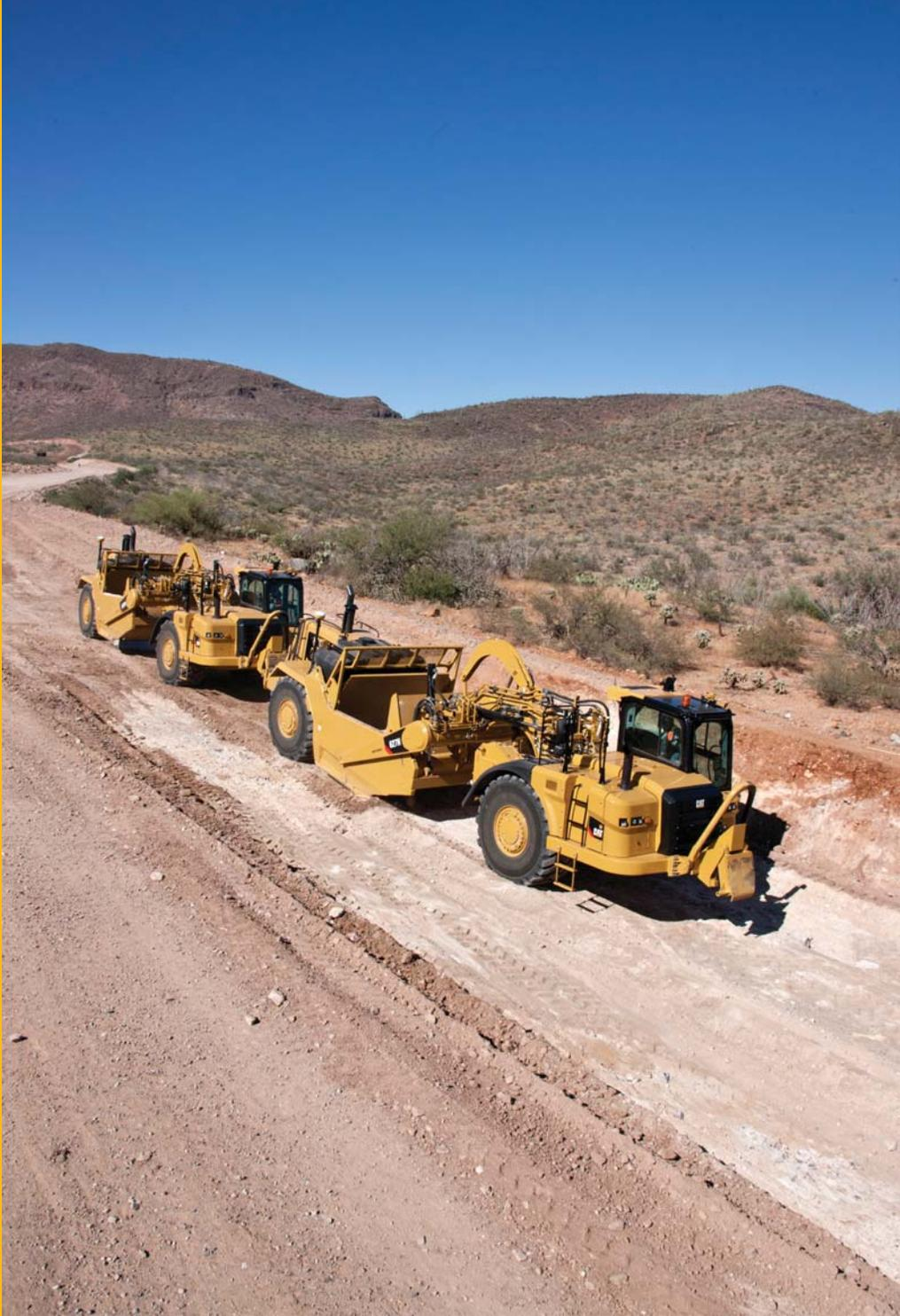
**Quick loading, high travel speeds and the ability to load and dump on the run yield fast cycle times, allowing Cat Wheel Tractor-Scrapers to consistently deliver high productivity at the lowest cost per ton.**
