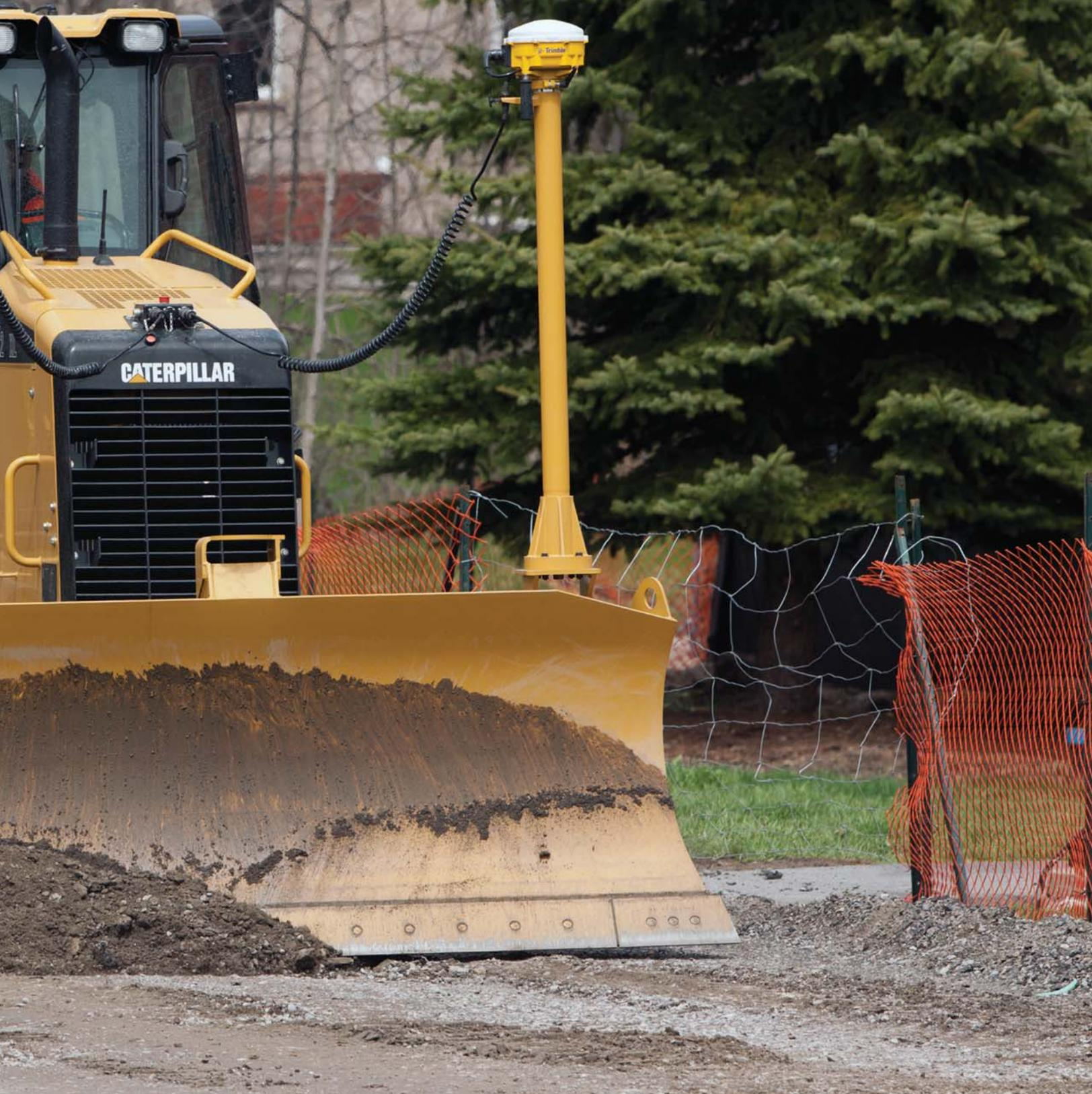
**Experience the most intuitive finish grading tractor in the industry. The Cat® D4K2 Track-Type Tractor with Stable Blade delivers a smooth finish grade with less operator effort. Stable Blade senses ground conditions and works with the operator to produce the desired grade. The addition of the integrated AccuGrade™ grade control system helps you get to target grade even faster, with fewer passes and less manpower. From the first cut to finish grade, the D4K2 sets the standard.**
