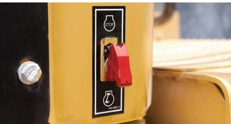
Your Cat G Series truck is designed to provide operators and technicians with easy access to common service points like engine lockout, machine system lockout, fluid level sight gauges, grease fittings and access to the engine for regularly scheduled maintenance.
