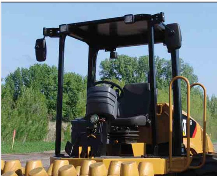
**Standard equipment.** Standard equipment includes two front-facing and two rear-facing working lights, hand rails with angled foot rests, a lockable vandalism guard and a rear view mirror.
