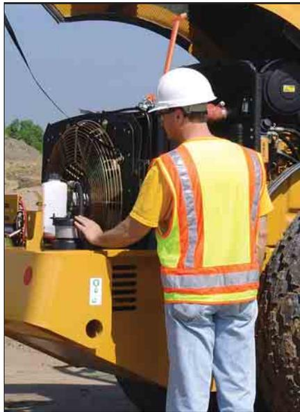
*The one-piece fiberglass hood tilts forward for exceptional access to the engine and cooling system. Daily service points are accessible from ground level and are grouped on one side of the machine.*
