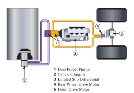
**Dual propel pumps.** Dual propel pumps provide separate, balanced hydraulic flow to the rear wheel axle and the drum drive motors. Provides superior gradeability on steep slopes and increases tractive effort in loose or poor underfoot conditions.
