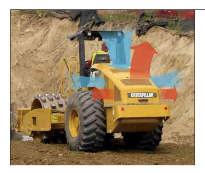
**Optimized air flow.** Pulls cool air from the middle of the hood and discharges hot air out the rear.
