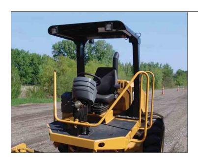
**Standard equipment.** Includes two front-facing and two rear-facing working lights, hand rails with angled foot rests, a lockable vandalism guard and a rear view mirror.
