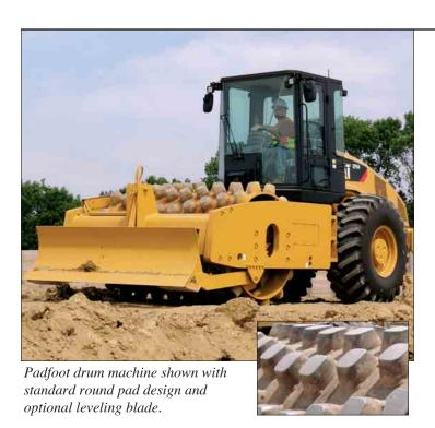
**Padfoot drum.** The padfoot drum has 140 pads welded on the drum in a chevron arrangement.
