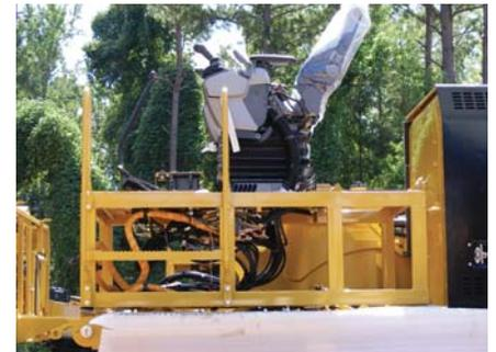
**Less-Off Cab.** A version of the 325D FM Log Loader is available less-off the cab to allow various AEM cabs to be installed by the dealer to meet regional customer needs.
