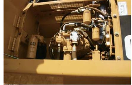
**Ground Level Service.** The design and layout of the 325D FM was made with the service technician in mind. Many service locations are easily accessible at ground level allowing critical maintenance to get done quickly and efficiently.
