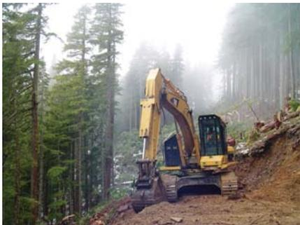
**Cat Roadbuilders.** The General Forestry model can be equipped with buckets, thumbs, clamshells and clearing grapples to fit a wide range of forest road building jobs.
