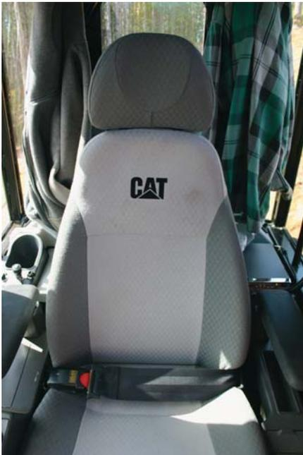
**Seat.** An air ride seat provides a variety of adjustments to suit the operator's size and weight including fore/aft, height and weight. Wide adjustable armrests and a retractable seat belt are also included.
