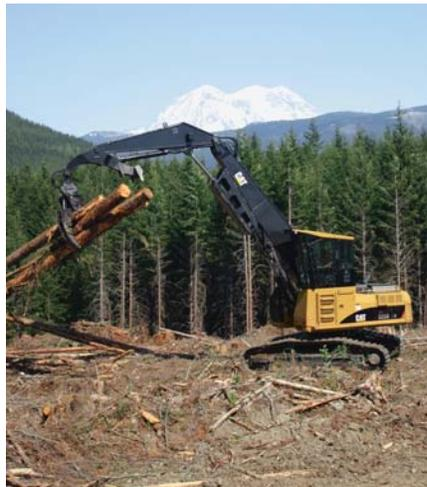
**Butt-N-Top.** The 325D FM can be shipped from the factory with an optional hydraulic arrangement and controls for AEM Butt-N-Top grapple installation, and an 11.3 m (37 ft) front.
