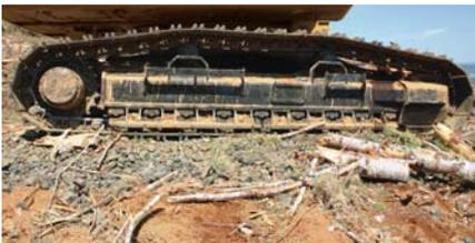
**Heavy-Duty Track Rollers.** Nine heavy-duty track rollers per side stand up to the toughest forest applications. Features include greater sealability, higher resistance to deformation and greater load carrying capacity.
