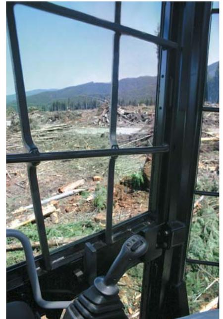
**Viewing.** Cab design optimizes post structures, and scratch-resistant polycarbonate window placement to provide excellent operator visibility to front, sides and rear. Forestry cab is designed with heavy-duty guarding, meeting all ROPS/FOPS/OPS/FOGS/TOPS and CB requirements. Windshield wipers are standard equipment on the FM cab.
