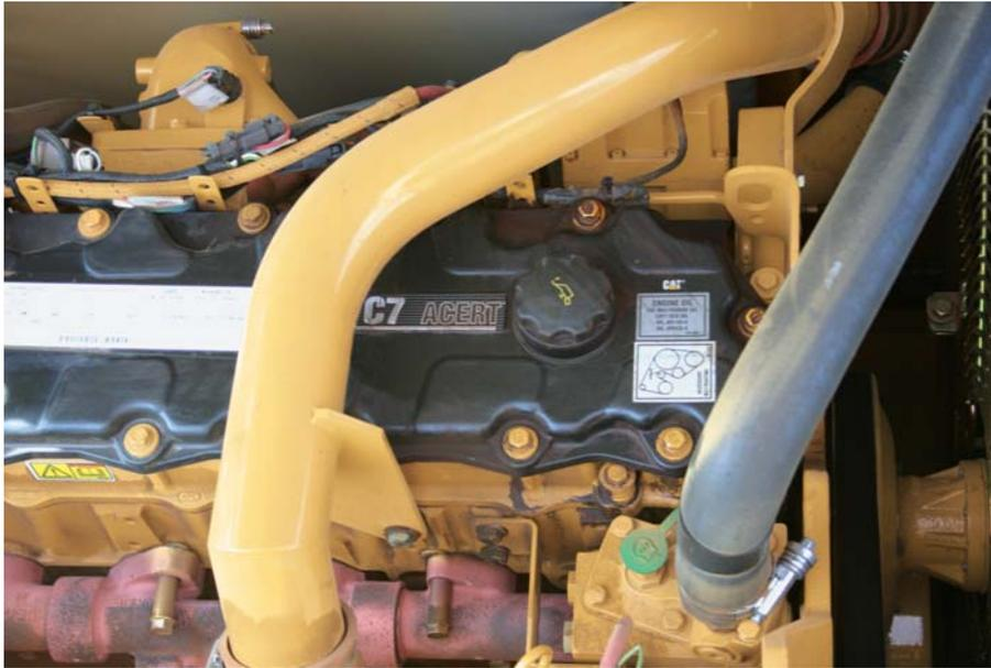
**Cat C7 ACERT™.** The Cat® C7 with ACERT™ Technology gives the 325D FM exceptional power and fuel efficiency unmatched in the industry, and provides high performance in all forestry applications. The C7 meets U.S. EPA emissions requirements.
