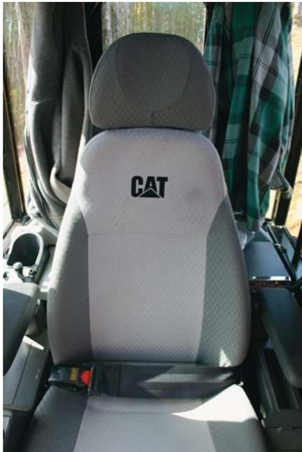
**Seat.** Air ride seat provides a variety of adjustments to suit the operator's size and weight including fore/aft, height and weight. Wide adjustable armrests and a retractable seat belt are also included.
