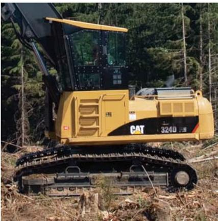
**Heavy-Duty Track Rollers.** Heavy-duty track rollers stand up to the toughest forest applications. Features include greater sealability, higher resistance to deformation and greater load carrying capacity.
