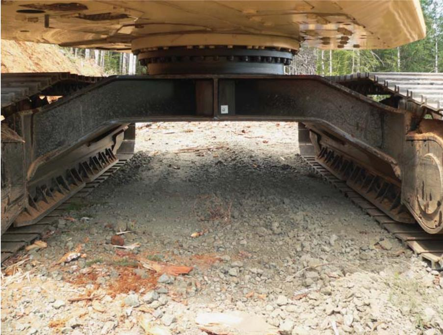
**Heavy-Duty Top Rollers.** Track rollers with dual supports replace standard single post mounted carrier rollers to assure superior endurance.
