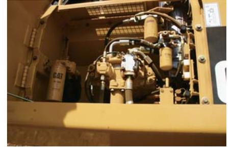
**Capsule Filter.** The hydraulic return filter, a capsule filter, is situated outside the hydraulic tank. This filter prevents contaminants from entering the system when hydraulic oil is changed and keeps the operation clean.
