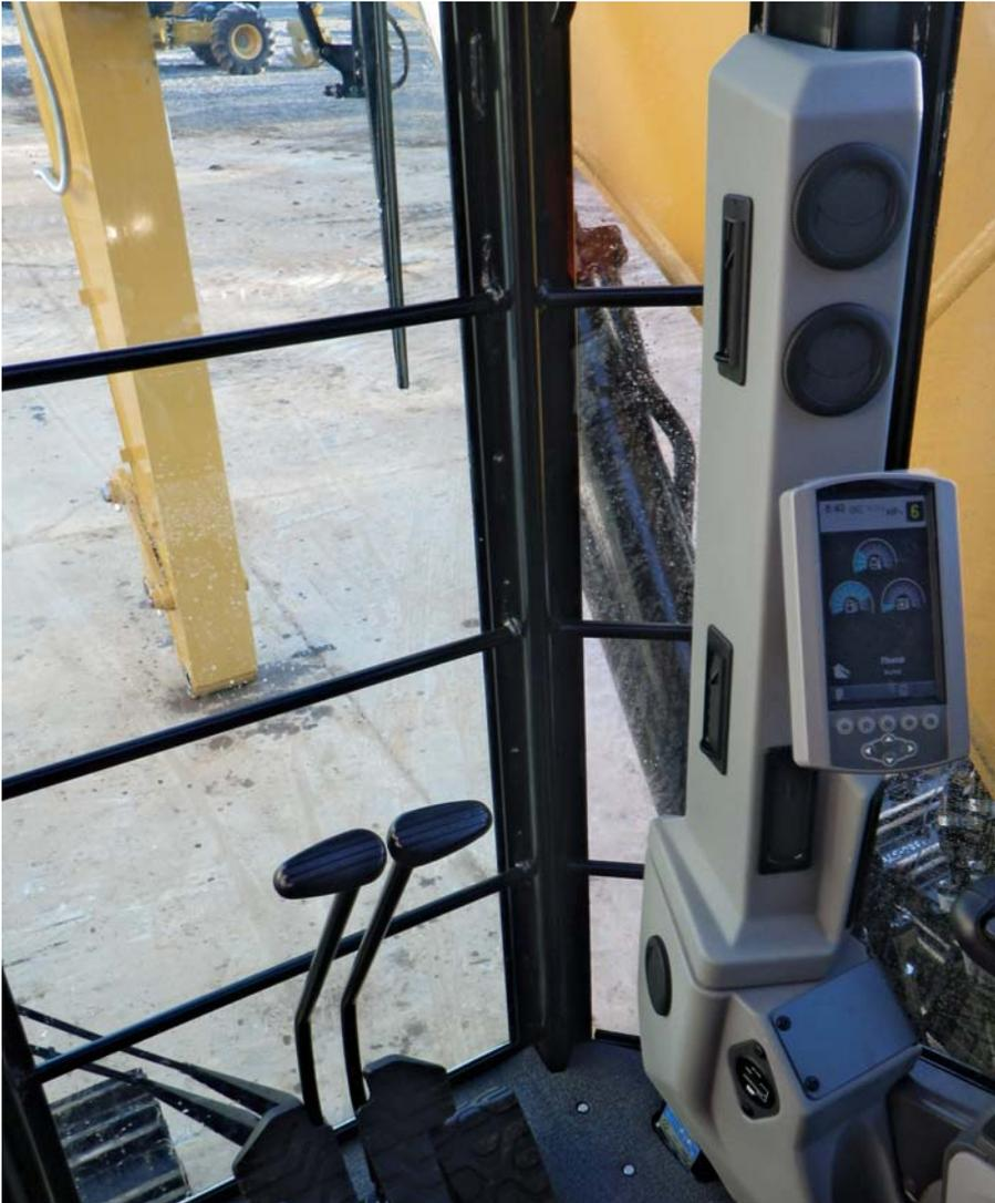
**Climate Control.** Positive filtered ventilation, a pressurized cab with bi-level air conditioner, heater and defroster keep operator comfortable in all types of weather conditions. Cab also has a forced air fan and a large fresh air window.
