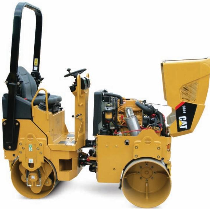
**Engine Enclosure.** Fiberglass engine enclosure pivots upward and locks open with a prop rod.
