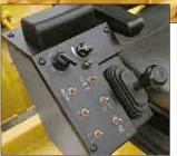
The side console features a padded arm rest, four-mode steering switch, speed control dial, propel lever, rotor elevation, front and rear rotor hood door switches, rear steering switch and sliding operator's station switch.
