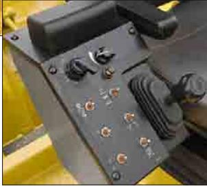
*The side console features a padded arm rest, the four mode steering switch, speed control dial, propel lever, rotor elevation, front and rear rotor hood door switches, rear steering switch and sliding operator's station switch.*
