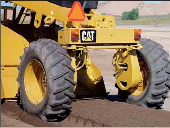
**Two propel pump system.** One pump is dedicated to drive the front wheels, while the second propel pump is dedicated to drive the rear wheels.
